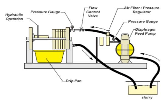
Companies use a Neoflux diaphragm pump to charge a filter press with Brine Water oil/sludge or Acidic Fluids.
